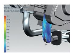
After using the flexible modes in a motion calculation, structural results can be visualized by animating the motion of the complete mechanism with the exact deformation of flexible bodies at any simulation time step, as well as the distribution of structural results in each flexible body such as strains, stresses and more.
