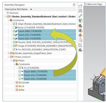
Position Override moves the Constraints into the Assembly active document, allowing the user to reposition the geometry
